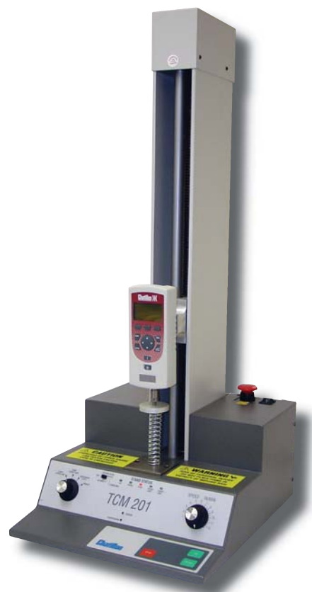
E-DFE shown with a TCD Digital Tester
